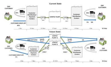
Most of the time savings were to be realized by creating a Finished Good 'Supermarket', which is a group of pre-sized FIFO lanes to facilitate the movement of finished good parts.
